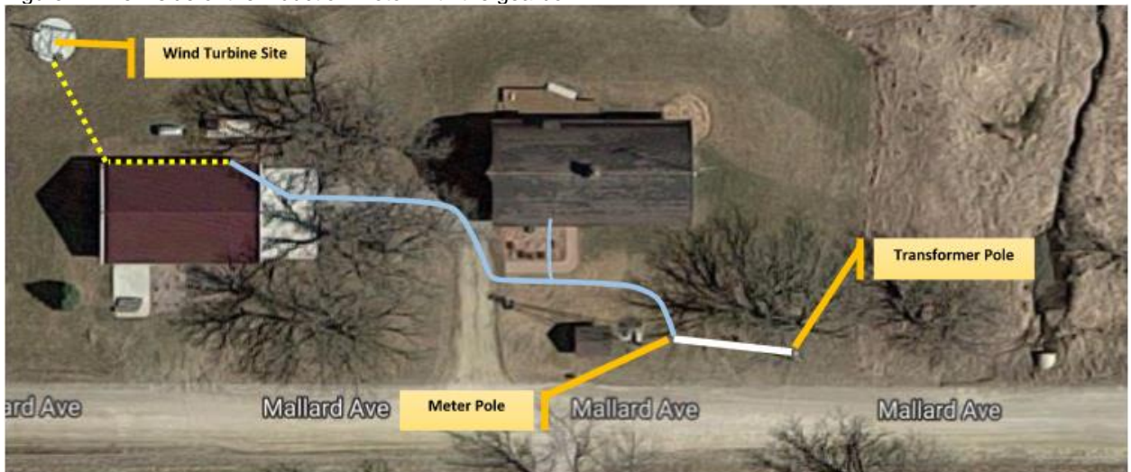
Figure 2- The placement of the wind turbine and the connecting wires to the electric grid.
