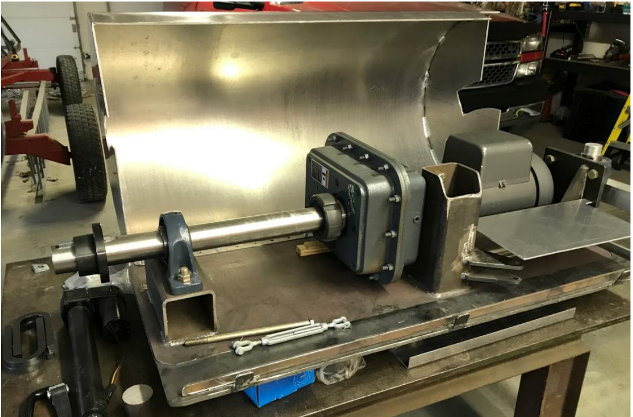
Figure 1- The inside of the induction motor with the gearbox
